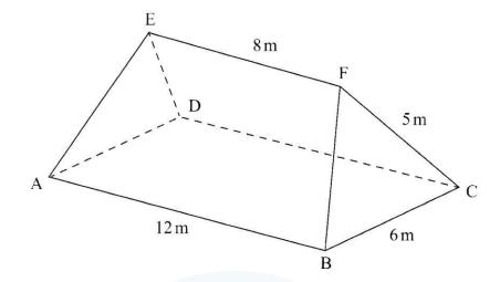
(a) Calculate, correct to 2 decimal places, the perpendicular distance of EF from the plane ABCD. (4 marks)
